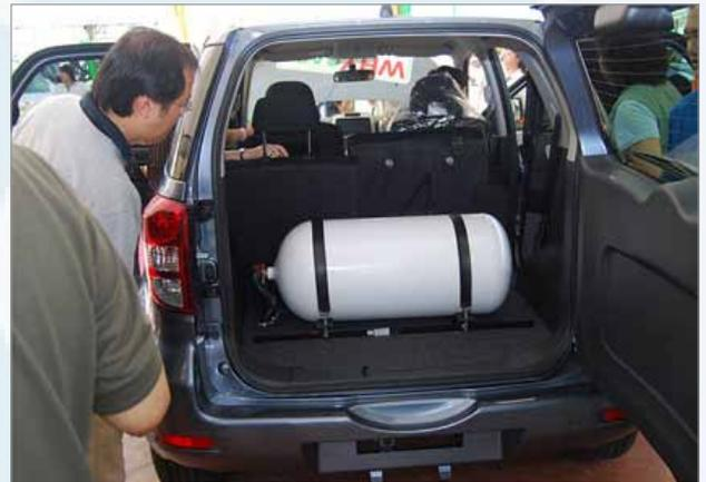
Onboard CNG Tank
